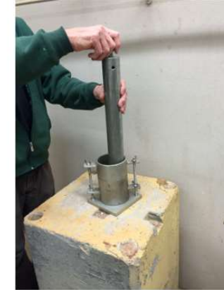
Standard Proctor /Modified Proctor One-Point Tests ASTM D698 / D1557
